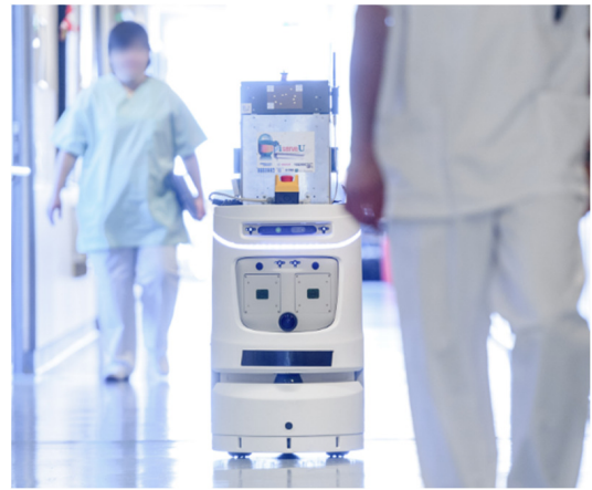
Figure 5. iserveU evaluation using a Robotino3 platform connected to the reference architecture via the SmartSoft (Schlegel et al. 2011) robotics middleware.
